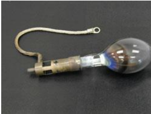
Hermetic seal failure
