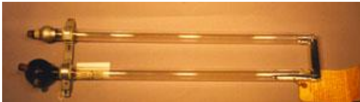
Electric discharge lamp invented by Hewitt in 1901
